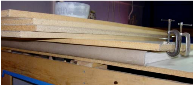
Make shift press to adhere flanges in the split boards.
