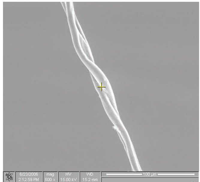
Figure 1: ESEM picture of cotton ( Gossypium ) fiber along the lengthwise direction
