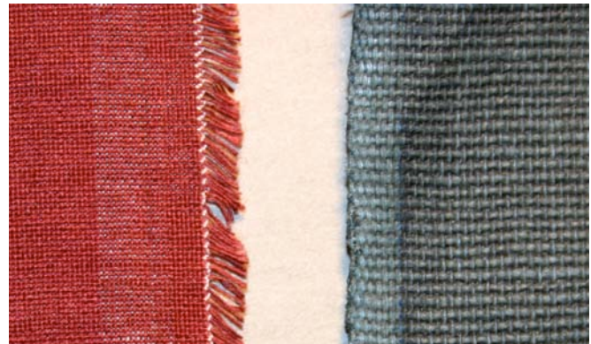
Figure 14: Two types of selvages on commercial book cloth. Left: shuttleless. Right: shuttle.
