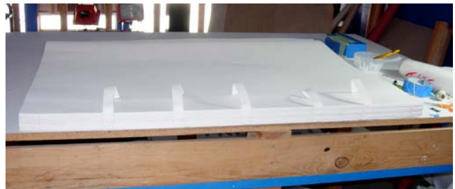
The book sewn on tapes, on the table edge used to tape the tapes underneath and sewn. A thin layer of PVA has been applied to the areas around the tapes.
