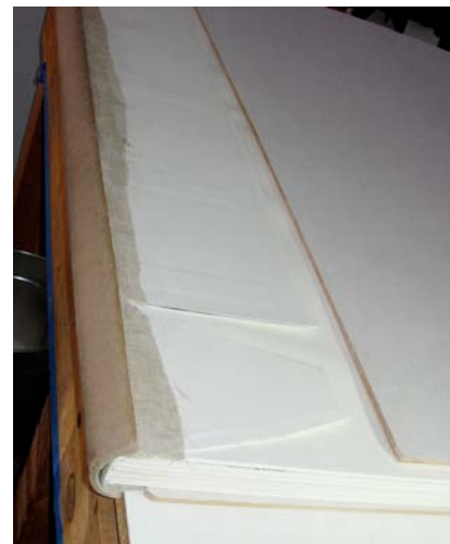
Attaching the split boards to the book, with flanges showing.
