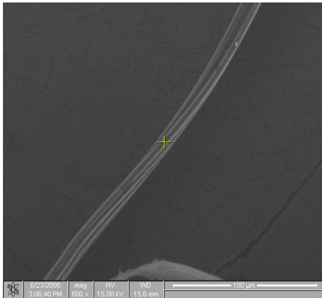
Figure 5: ESEM picture of rayon in the lengthwise direction.
