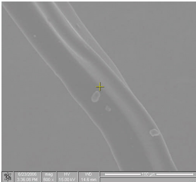
Figure 8: ESEM picture of nylon in the lengthwise direction.
