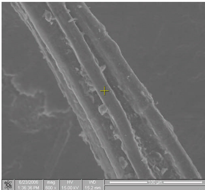
Figure 3: ESEM picture of hemp ( Cannabis sativa ) fiber along the lengthwise direction.
