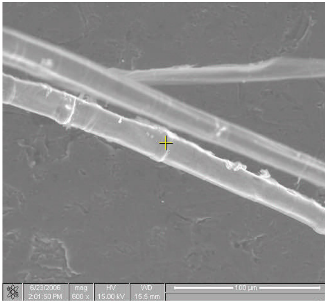
Figure 2: ESEM picture of flax ( Linum usitatissimum ) fiber along the lengthwise direction.
