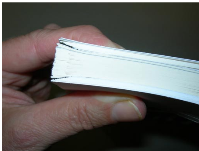
A special trim pad was needed to compensate for the swell at both the spine and fore-edge while trimming the head and tail of the book.
