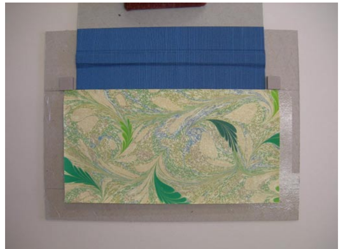
Craig Jensen's right angle jig set up using shop tools secured to a cutting mat. A similar set up can be made with binders' board.
