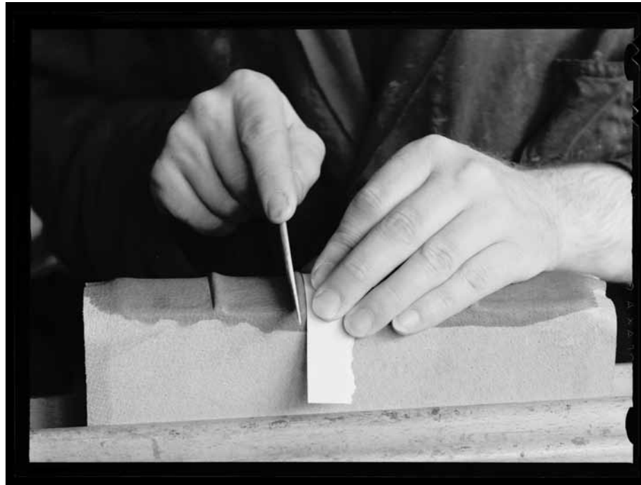
Applying leather to the spine of the book using a bone folder.
