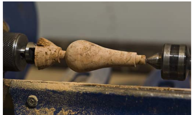
An awl handle on the lathe after shaping
